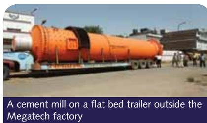
A cement mill on a flat bed trailer outside the Megatech factory
